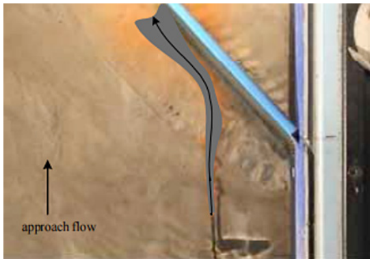
Fig. 3: Flow diversions towards the main channel from the upstream and the downstream of the modified bandal 10
