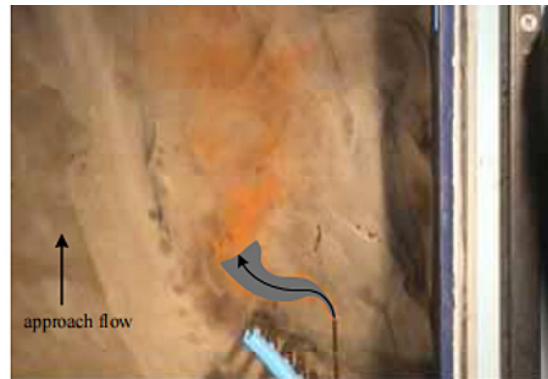
Fig. 3: Flow diversions towards the main channel from the upstream and the downstream of the modified bandal 10
